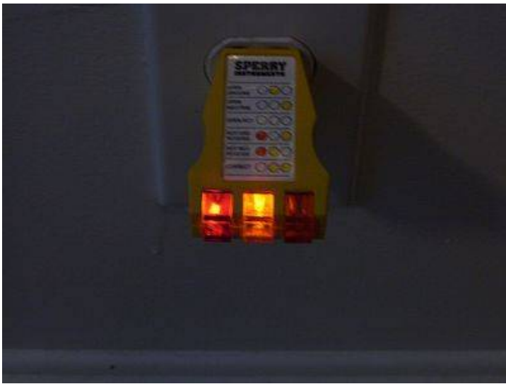
Photo 9 Reversed polarity (hot/neutral).
