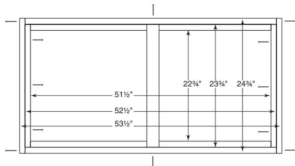
Assemble side pieces, end pieces, and brace as shown. The cover piece will drop in and be attached with adhesive and nails.
