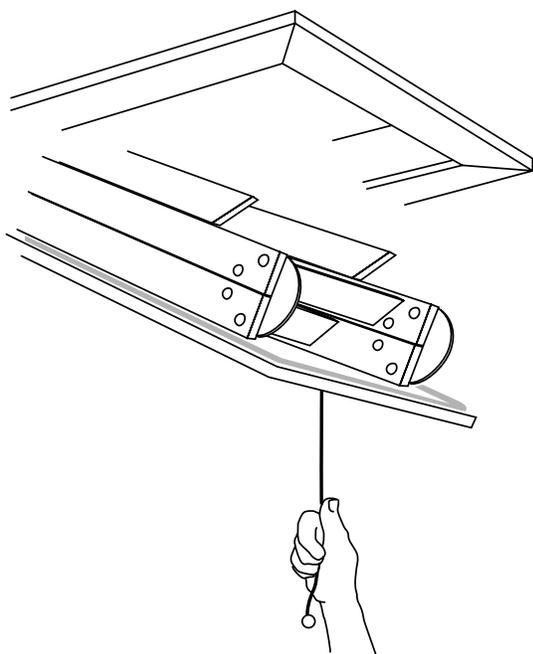
*An attic access is often a big hole in the thermal envelope of the house. Adding an insulated cover and weatherstripping to a pull-down stairs can reduce infiltration and heat loss through this passageway. Latch bolts (not shown) may be installed to help ensure a tighter seal.*
