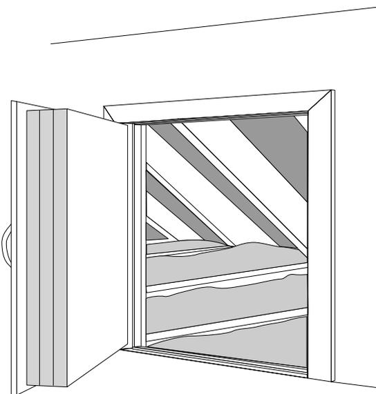
*Add R-value to the knee-wall door, by adhering rigid insulation board (sandwiched together with construction adhesive and screws) to the back of the door. The clearance between the insulation and the door frame as well as air sealing details will require special attention.*
