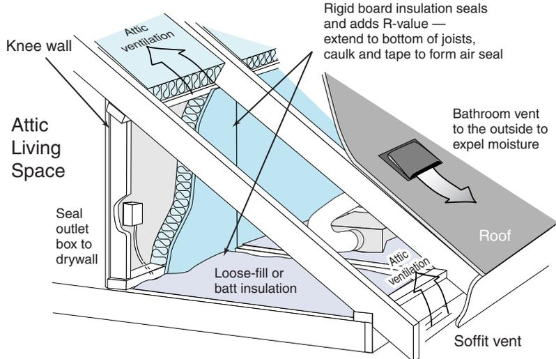
*The attic knee wall is often underinsulated and leaky. Install adequate insulation and air seal around the living space for continuity in the building envelope.*
