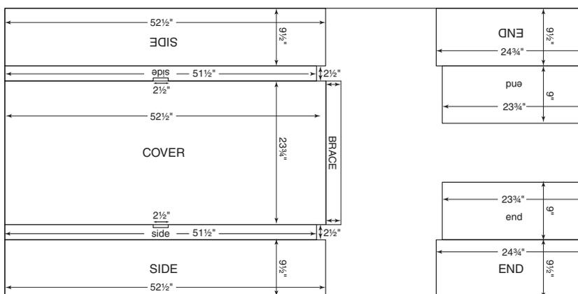
Dimensions shown are for a box 53 1/2" outside (51 1/2" inside), 24 3/4" outside (22 3/4" inside), and 9" of depth inside. Adjust dimensions to fit the specific stairs being installed.
